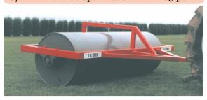
920mm(36") DIAMETER 12mm PLATE 3.05m 70hp 1370Kg 3370Kg £4956 3.66m 80hp 1670Kg 4070Kg £5555 Optional Extra Scraper Blade £107 per m
