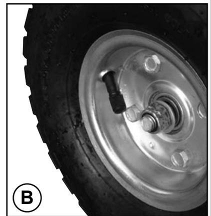
Flat washer and locknut are used on the outside of the wheel. Install the wheel with the valve stem to the outside.
