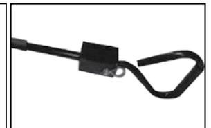
Handle can be removed to expose a pin connection that will attach to receiver of motorized vehicle. If hand grip is removed, place in a safe place for future use.
