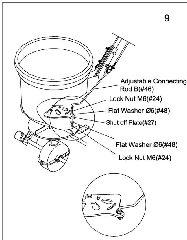
10. a) The three large holes at the bottom of the hopper should match the three holes in the adjustable plate. If they match, do nothing. If they do not match, push the handle down to the lowest position and adjust the positions of the two nuts on the threaded control bar until the three holes match up. If the holes are not properly aligned, the hopper will not close completely.
